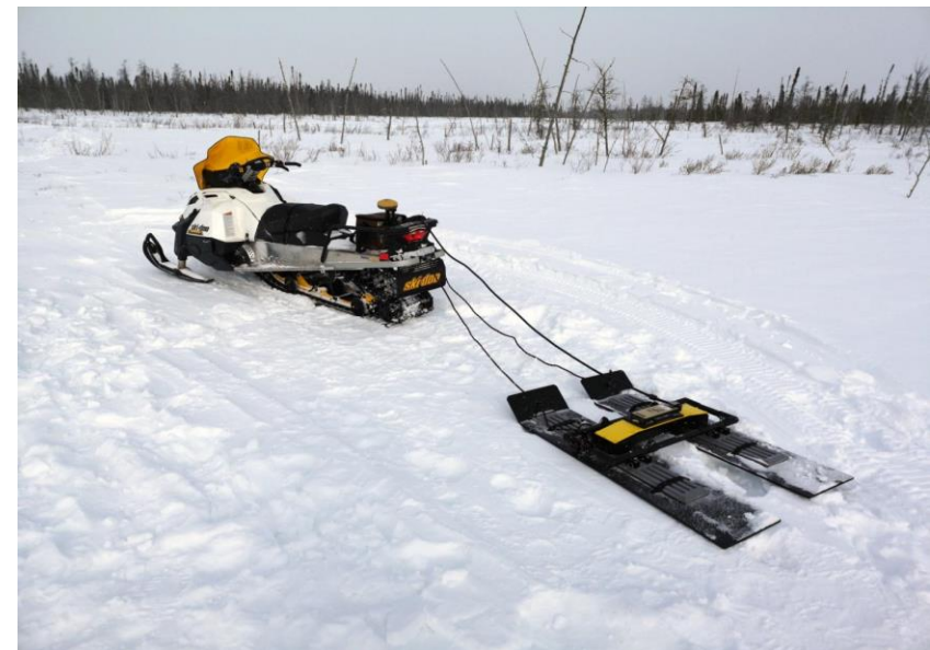
February 22, 2019: GPR 100MHz transmitter/receiver setup mounted on skis and pulled by snowmobile
