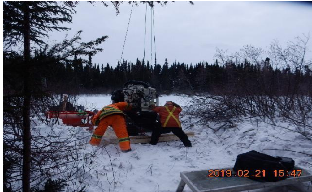
February 21, 2019: Drill rig slung by helicopter being placed on drilling platform.
