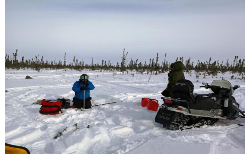
February 19, 2019: Using a peat probe to verify organic thickness at one of the survey sites
